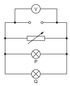
The resistance of the variable resistor is increased. The voltmeter reading remains unchanged.
